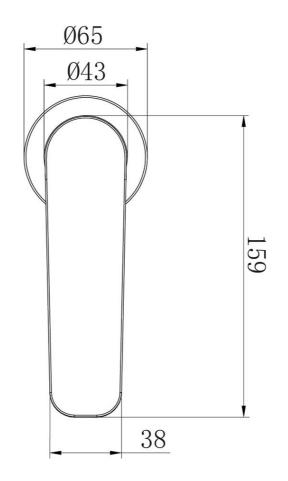
Note: All dimensions are in millimetres and are subject to normal manufacturing variations. Always use the physical product measurements for cut-outs and rough-ins as the technical details shown may differ from the actual product. Use acetic cured silicone sealant. Do not use epoxy type adhesives. Clean with damp cloth. Do not use abrasive cleaners, liquids or pastes.
