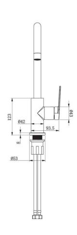
Note: All dimensions are in millimetres and are subject to normal manufacturing variations. Always use the physical product measurements for cut-outs and rough-ins as the technical details shown may differ from the actual product. Use acetic cured silicone sealant. Do not use epoxy type adhesives. Clean with damp cloth. Do not use abrasive cleaners, liquids or pastes.
