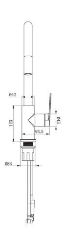
Note: All dimensions are in millimetres and are subject to normal manufacturing variations. Always use the physical product measurements for cut-outs and rough-ins as the technical details shown may differ from the actual product. Use acetic cured silicone sealant. Do not use epoxy type adhesives. Clean with damp cloth. Do not use abrasive cleaners, liquids or pastes.
