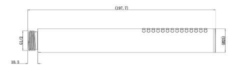
Note: All dimensions are in millimetres and are subject to normal manufacturing variations. Always use the physical product measurements for cut-outs and rough-ins as the technical details shown may differ from the actual product. Use acetic cured silicone sealant. Do not use epoxy type adhesives. Clean with damp cloth. Do not use abrasive cleaners, liquids or pastes.
