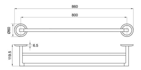
Note: All dimensions are in millimetres and are subject to normal manufacturing variations. It is recommended to use the physical product measurements for cut-outs and rough-ins as the technical details shown may differ from the actual product. Use acetic cured silicone sealant. Do not use epoxy type adhesives. Clean with damp cloth. Do not use abrasive cleaners, liquids or pastes.
