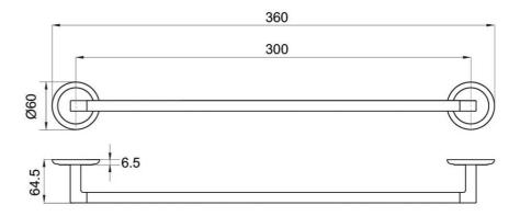
Note: All dimensions are in millimetres and are subject to normal manufacturing variations. It is reccommended to use the physical product measurements for cut-outs and rough-ins as the technical details shown may differ from the actual product. Use acetic cured silicone sealant. Do not use epoxy type adhesives. Clean with damp cloth. Do not use abrasive cleaners, liquids or pastes.
