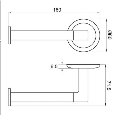
Note: All dimensions are in millimetres and are subject to normal manufacturing variations. It is reccommended to use the physical product measurements for cut-outs and rough-ins as the technical details shown may differ from the actual product. Use acetic cured silicone sealant. Do not use epoxy type adhesives. Clean with damp cloth. Do not use abrasive cleaners, liquids or pastes.
