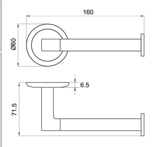
Note: All dimensions are in millimetres and are subject to normal manufacturing variations. It is reccommended to use the physical product measurements for cut-outs and rough-ins as the technical details shown may differ from the actual product. Use acetic cured silicone sealant. Do not use epoxy type adhesives. Clean with damp cloth. Do not use abrasive cleaners, liquids or pastes.
