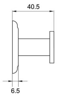
Note: All dimensions are in millimetres and are subject to normal manufacturing variations. It is reccommended to use the physical product measurements for cut-outs and rough-ins as the technical details shown may differ from the actual product. Use acetic cured silicone sealant. Do not use epoxy type adhesives. Clean with damp cloth. Do not use abrasive cleaners, liquids or pastes.
