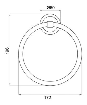
Note: All dimensions are in millimetres and are subject to normal manufacturing variations. It is reccommended to use the physical product measurements for cut-outs and rough-ins as the technical details shown may differ from the actual product. Use acetic cured silicone sealant. Do not use epoxy type adhesives. Clean with damp cloth. Do not use abrasive cleaners, liquids or pastes.
