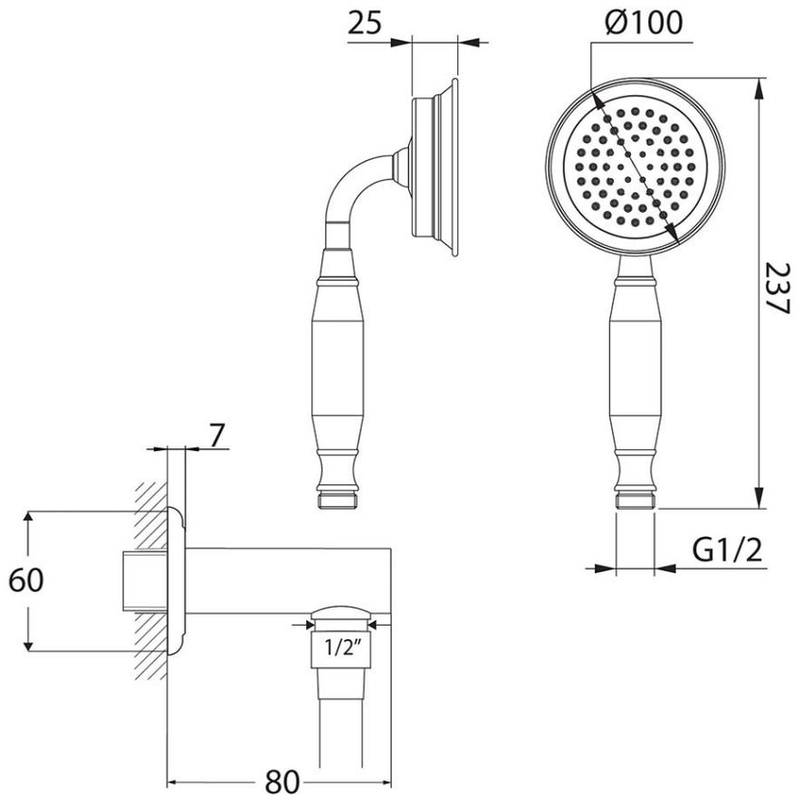
Note: All dimensions are in millimetres and are subject to normal manufacturing variations. It is recommended to use the physical product measurements for cut-outs and rough-ins as the technical details shown may differ from the actual product. Use acetic cured silicone sealant. Do not use epoxy type adhesives. Clean with damp cloth. Do not use abrasive cleaners, liquids or pastes.
