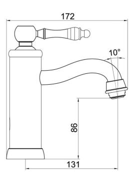
Note: All dimensions are in millimetres and are subject to normal manufacturing variations. It is reccommended to use the physical product measurements for cut-outs and rough-ins as the technical details shown may differ from the actual product. Use acetic cured silicone sealant. Do not use epoxy type adhesives. Clean with damp cloth. Do not use abrasive cleaners, liquids or pastes.
