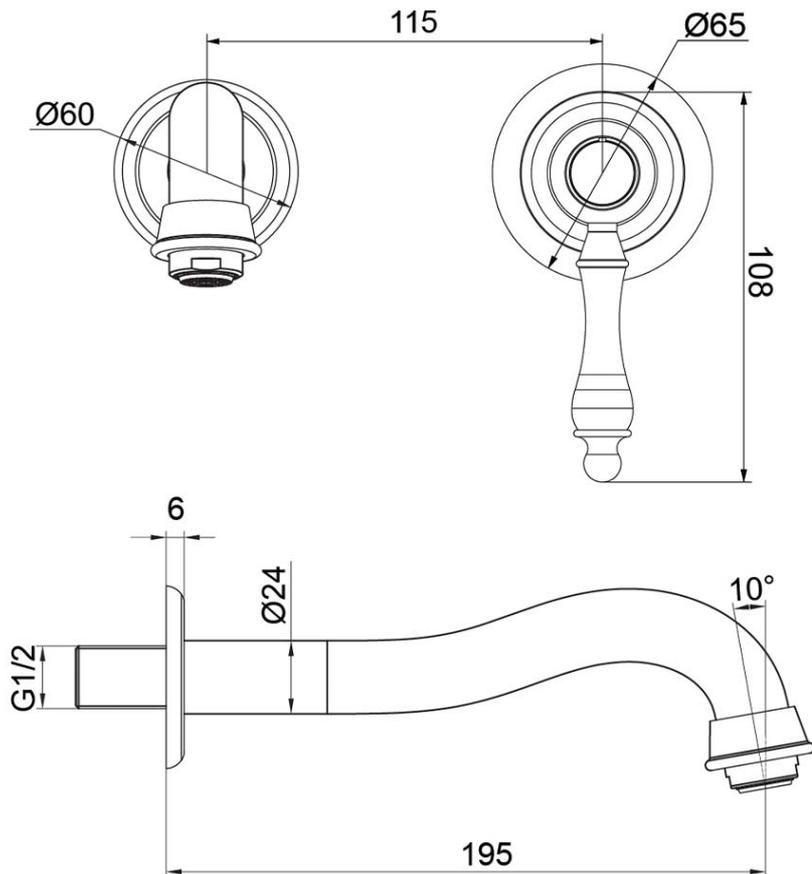
*Note: All dimensions are in millimeters and are subject to normal manufacturing variations. It is recommended to use the physical product measurements for cut-outs and rough-ins as the technical details shown may differ from the actual product. Use acetec cured silicone sealant. Do not use epoxy type adhesives. Clean with damp cloth. Do not use abrasive cleaners, liquids or pastes.*
