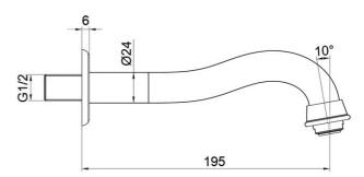
Note: All dimensions are in millimetres and are subject to normal manufacturing variations. It is reccommended to use the physical product measurements for cut-outs and rough-ins as the technical details shown may differ from the actual product. Use acetic cured silicone sealant. Do not use epoxy type adhesives. Clean with damp cloth. Do not use abrasive cleaners, liquids or pastes.
