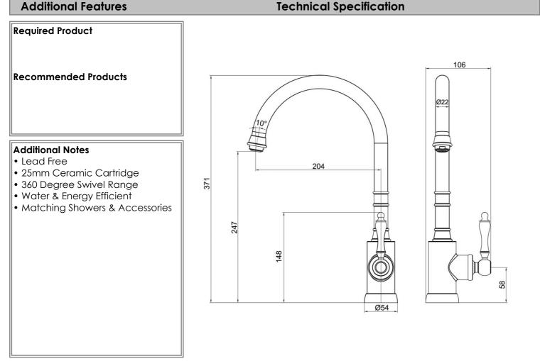
Note: All dimensions are in millimetres and are subject to normal manufacturing variations. It is reccommended to use the physical product measurements for cut-outs and rough-ins as the technical details shown may differ from the actual product. Use acetic cured silicone sealant. Do not use epoxy type adhesives. Clean with damp cloth. Do not use abrasive cleaners, liquids or pastes.
