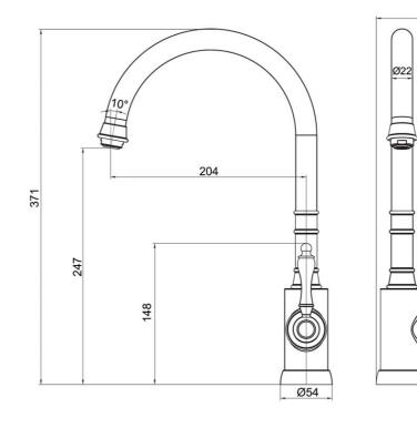
Note: All dimensions are in millimetres and are subject to normal manufacturing variations. It is reccommended to use the physical product measurements for cut-outs and rough-ins as the technical details shown may differ from the actual product. Use acetic cured silicone sealant. Do not use epoxy type adhesives. Clean with damp cloth. Do not use abrasive cleaners, liquids or pastes.
