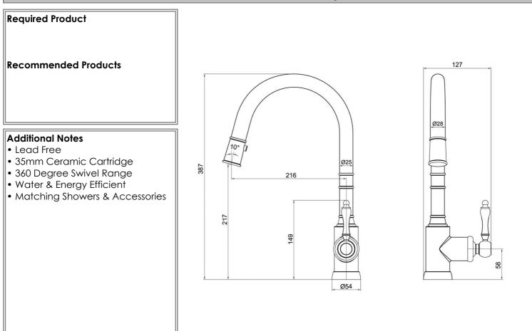
Note: All dimensions are in millimetres and are subject to normal manufacturing variations. It is reccommended to use the physical product measurements for cut-outs and rough-ins as the technical details shown may differ from the actual product. Use acetic cured silicone sealant. Do not use epoxy type adhesives. Clean with damp cloth. Do not use abrasive cleaners, liquids or pastes.
