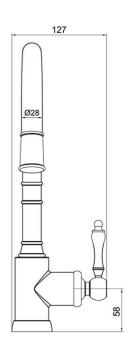
Note: All dimensions are in millimetres and are subject to normal manufacturing variations. It is reccommended to use the physical product measurements for cut-outs and rough-ins as the technical details shown may differ from the actual product. Use acetic cured silicone sealant. Do not use epoxy type adhesives. Clean with damp cloth. Do not use abrasive cleaners, liquids or pastes.
