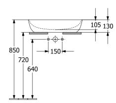
Note: All dimensions are in millimetres and are subject to normal manufacturing variations. Always use the physical product measurements for cut-outs and rough-ins as the technical details shown may differ from the actual product. Use acetic cured silicone sealant. Do not use epoxy type adhesives. Clean with damp cloth. Do not use abrasive cleaners, liquids or pastes.
